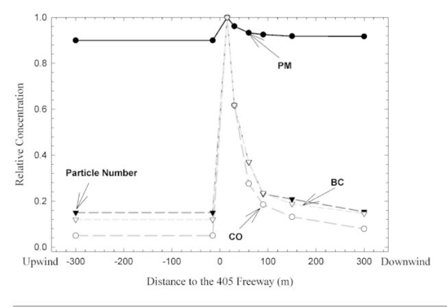
Fig 5.6 Proximity to traffic (60, 90, and 300 m). While  $PM_{2.5}$  varies very little (5–10%), ultrafine particles, black carbon (BC), and carbon monoxide (CO) decrease within 100 m to < 20%.
