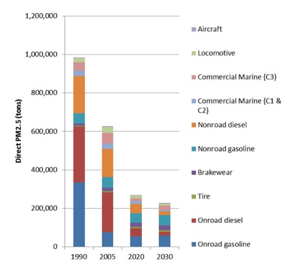
C1, commercial marine engines < 5 liters/cylinder; C2, commercial marine engines 5–30 liters/cylinder; C3, commercial marine engines > 30 liters/cylinder. Reproduced from EPA (2012).
