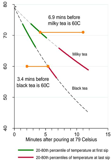
\*Medium temperature at pouring, 79 Celsius. Cooling curve for ambient temperature of 20C
